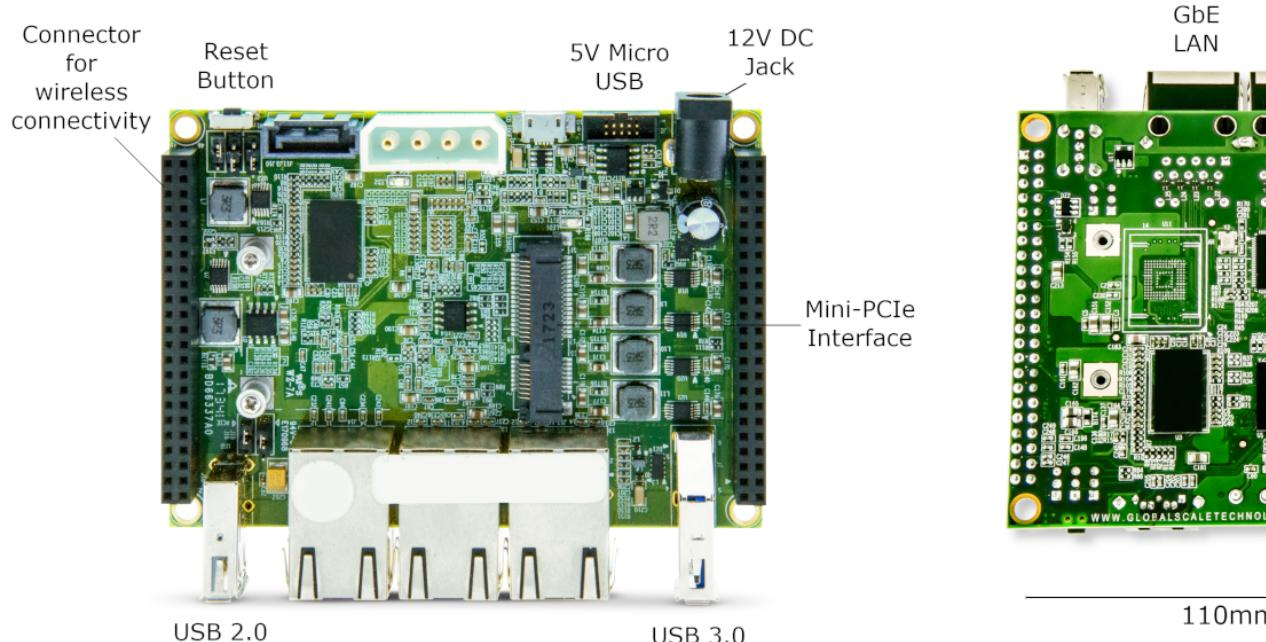
Note: Graphic shows Gateway without extension board and wireless module.
