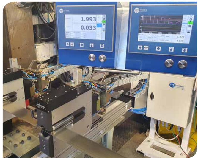
Tenneco, Italy, bimetetal, rolling mill - Single line gauge + scanning head
