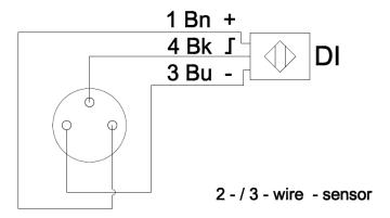
b) Output signal – 1 connector connects 1 digital output, FEEC-0404P-M8, FEEC-08UP-M8 support this connection.
